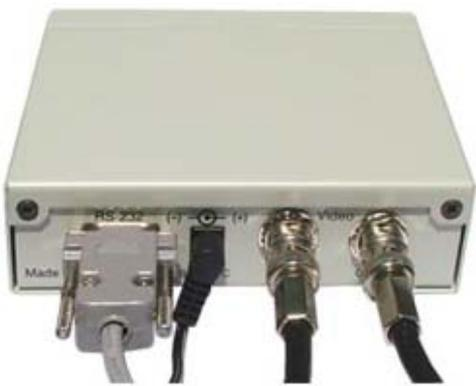
Figure 3: VSI-Pro-IBM Cable Connections
